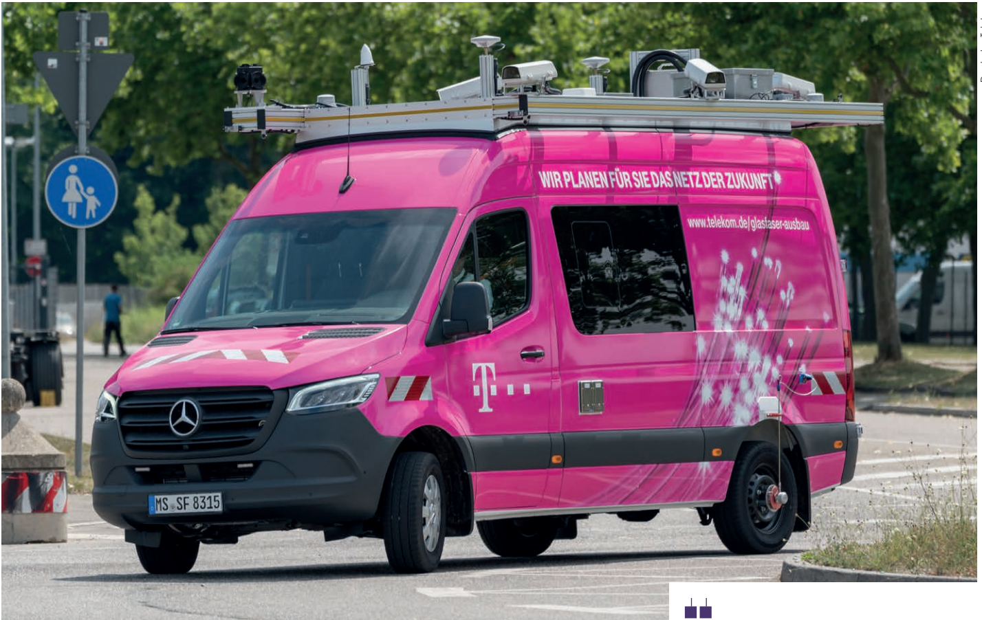
Deutsche Telekom's T-Cars can optimise land surveying and make sure that laying routes are as short and simple as possible when expanding the network
